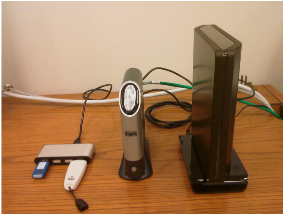
Figure 3: The RRD prototype, consisting of a Linksys NSLU2 storage link, a Seagate Free Agent Pro external hard drive, and a USB flash memory drive, connected to a hub for clarity. A token is plugged into the leftmost spot on the USB hub.
